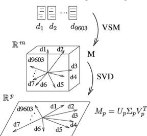
Fig. 1. Vectors in the VSM are projected to the reduced space by using SVD.
