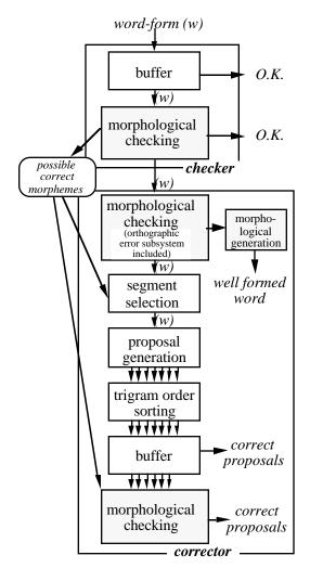
Fig. 2 Architecture of the checker/corrector
